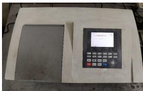
Figure 3.11. UV- visible spectrophotometer used for determining vanadium peaks.
